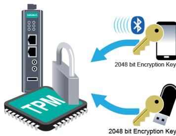
For example, Arm-based computers that support TPM v2.0. Bringing TPM and Arm-based computers together gives system integrators and industrial engineers a powerful new tool in their security arsenal. By creating a specific cryptographic key for each individual device, which is hardcoded within the platform itself, the data stored on the computing system is secured and protected from being read by an unauthorized party. Moreover, the OS on the system can be locked from being overwritten
