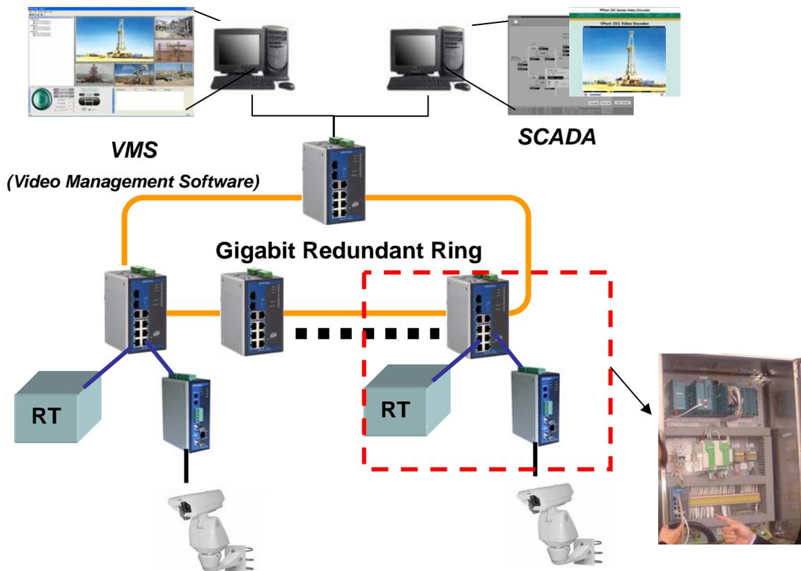
Video networking applications play a major role in helping SCADA administrators monitor field site situations using actual video images. Video management software is used to display the video images, which can also be displayed on the SCADA server when operators are faced with an emergency situation. By using actual video images, operators can know immediately what has happened at the field site, and then make the right decision on how to handle the problem.
