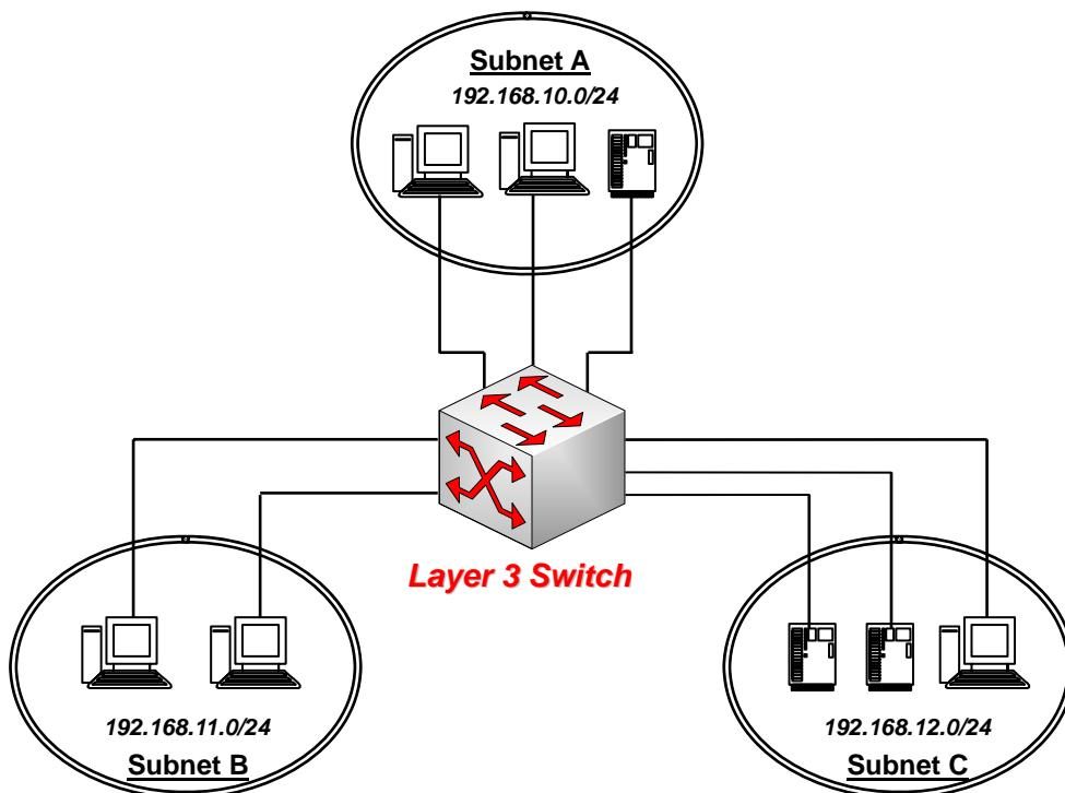
In the figure, we show a layer 3 switch connected to switches and hosts from the three subnets. Since the layer 3 switch uses IP addresses to direct traffic, it is capable of transmitting packets from any network host on the LAN to any other
