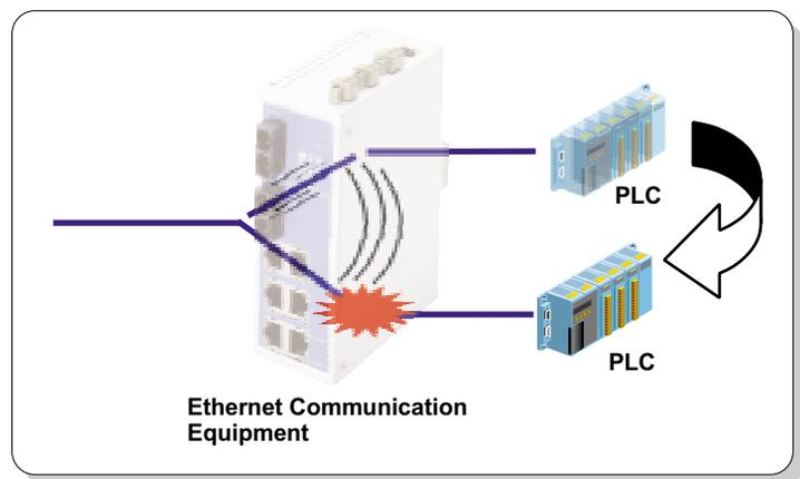
Another important consideration is that when industrial Ethernet communication equipment is used as part of an automation system, it is more often used to connect devices, as opposed to computer hosts. And since all automation systems incorporate sensitive devices that must be protected from unauthorized access, it is very important to have some type of authentication system set up that only allows authorized users to access the system.
