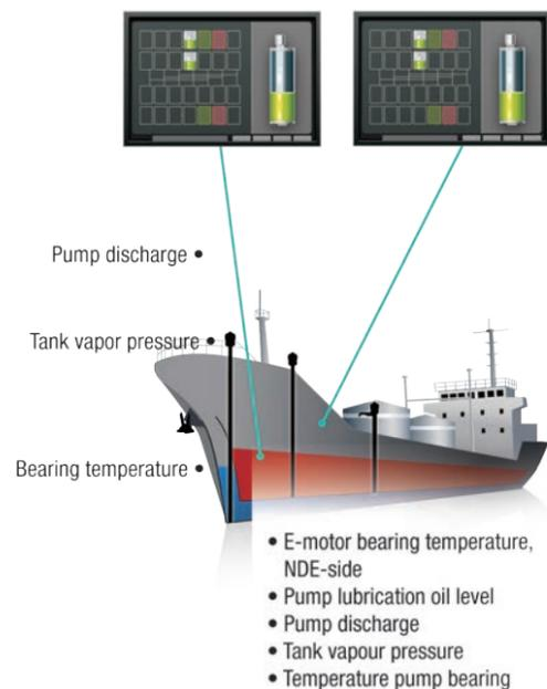
full alarms, and performance and sensor readings. Most remarkably, the pump will also be capable of direct communications with remote stations of any sort, whether onboard the ship, in distant central offices, or even with mobile stations only a kilometer or two away. As with so many other recent advances in maritime technology, the situational awareness and scope of access are unprecedented.
