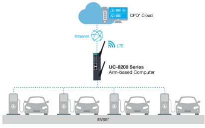
\*CPO: Charging Point Operator \*EVSE: Electric Vehicle Supply Equipment ---- Wireless
