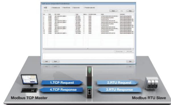
**Optimizing SCADA Systems Using a Modbus Gateway**
