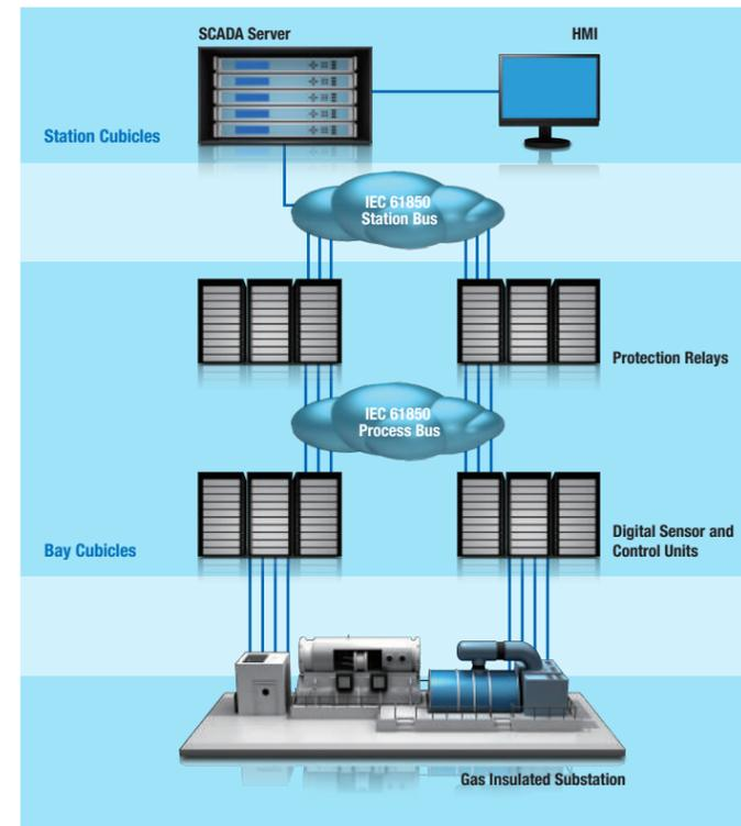
In 2005, the IEC 61850 standard was greatly improved by defining a Process Bus to connect the Process Level with the Bay Level.
