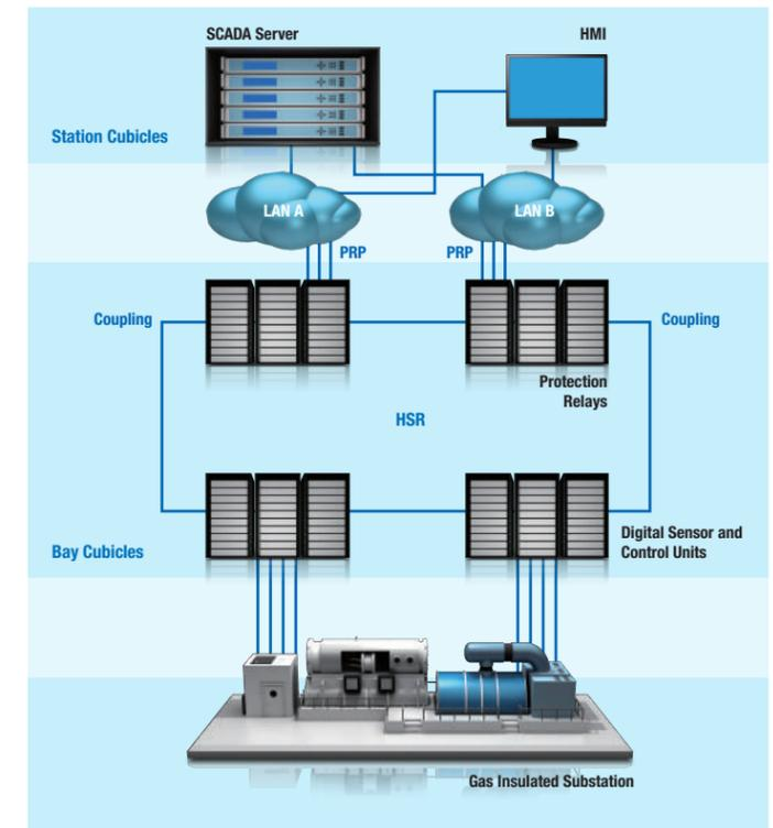
The latest development in the IEC 61850 standard was the inclusion of the PRP/HSR protocol in 2010. PRP/HSR (parallel redundancy protocol/high-availability seamless redundancy) specifies how to use two Ethernet networks to ensure seamless failover if one of the redundant networks fails.
