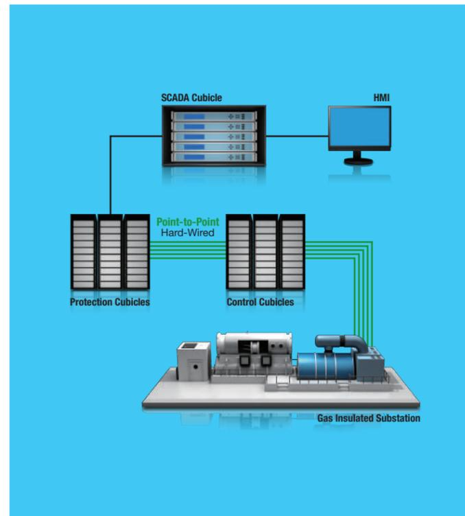
In the 1960's a conventional substation was rather bulky, with copper or fiber wiring used to hard-wire one device to another.
