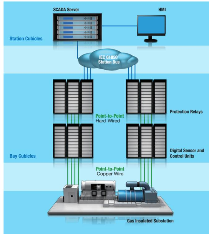
The release of the IEC 61850 Station Bus protocol in the 1980's was a big first step forward on the way to implementing a substation-wide all-purpose network.
