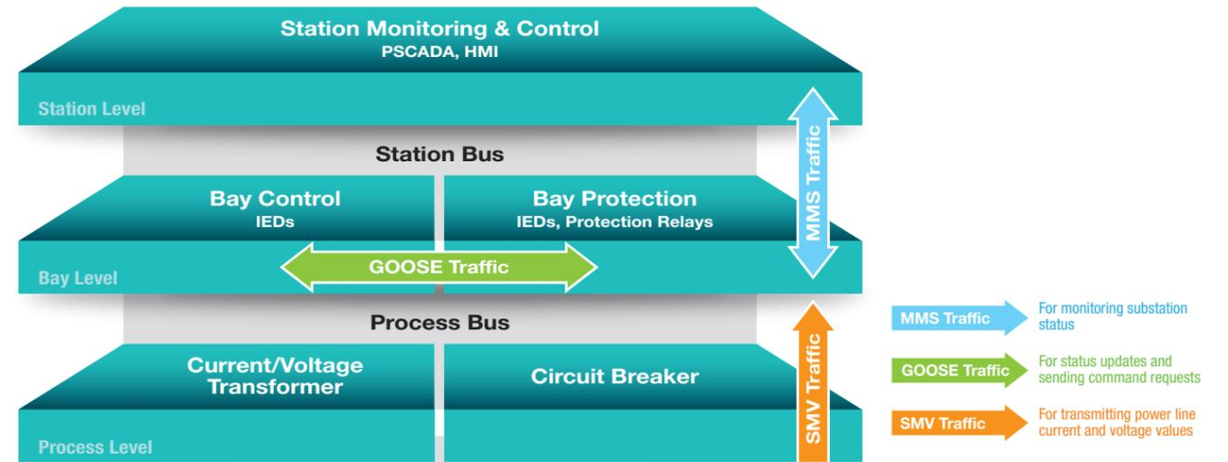
**The example in the following figure illustrates how the three protocols contribute to substation communication.**
