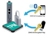
For example, Arm-based computers that support TPM v2.0. Bringing TPM and Armbased computers together gives system integrators and industrial engineers a powerful new tool in their security arsenal. By creating a specific cryptographic key for each individual device, which is hardcoded within the platform itself, the data stored on the computing system is secured and protected from being read by an unauthorized party. Moreover, the OS on the system can be locked from being overwritten
