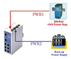
Furthermore, the system's hardware should at least be compatible with unregulated DC and have reverse power protection. As discussed next, the two most common ways to send power failure alarms to network administrators is by e-mail or relay output.
