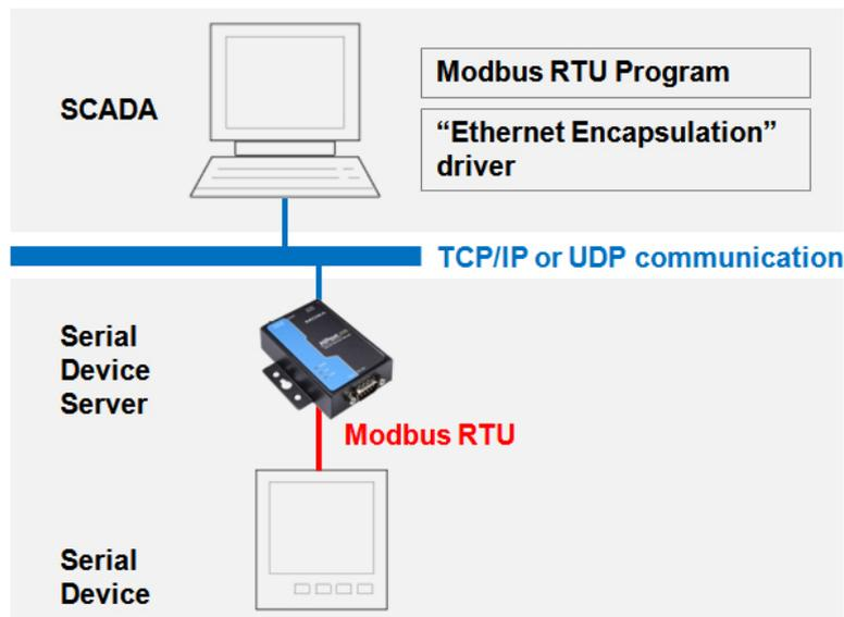
Although serial device servers can also connect Modbus RTU devices to an Ethernet network, a gateway solution can meet almost every system requirement. Your host must be able to support Modbus TCP connections. This shouldn't be a problem since Modbus TCP is very popular and already widely supported. Here are a few situations where you will need to use a designated gateway solution:
