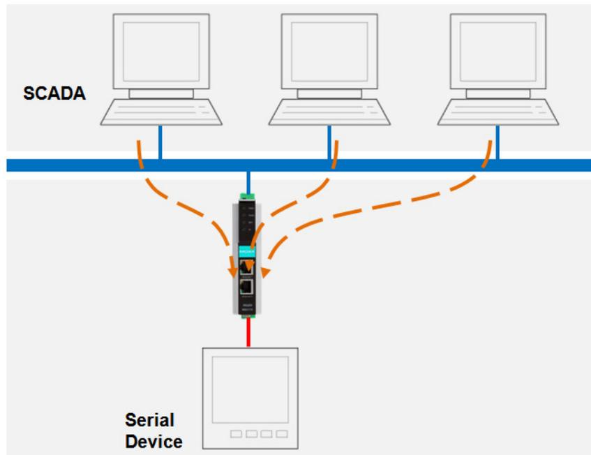
But, the above offering is not the only solution. Some gateways support an agent mode, which actively and continuously retrieves data from connected devices. The updated data is stored in internal memory, which is used to reply to host requests. Although this solution is faster and more efficient, the data retrieved might not be the most current in real time.
