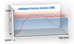
sensor (T-sensor). These enhancements allow the system to protect itself by shutting down hard drives when things get too hot (thereby eliminating a key heat contributor and protecting data), or by heating up storage devices when the device's ambient temperature drops to well below zero. Further, an independent T-sensor may also serve as a powerful supplementary tool for predictive maintenance (PdM) analysis of the local system.
